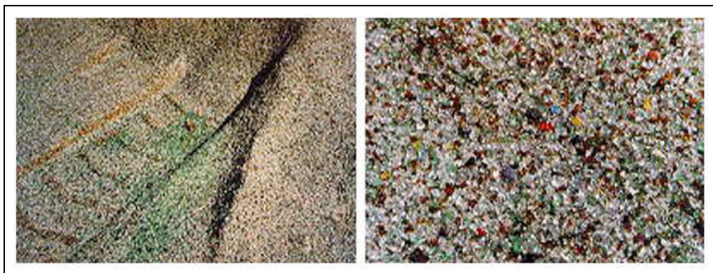
Figure 6: Recycled glass as aggregate in asphalt concrete
