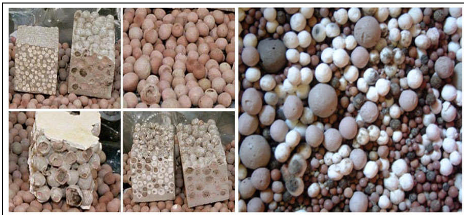
Figure 2: "Geofil Bubbles"- expanded glass aggregate for lightweight concrete
